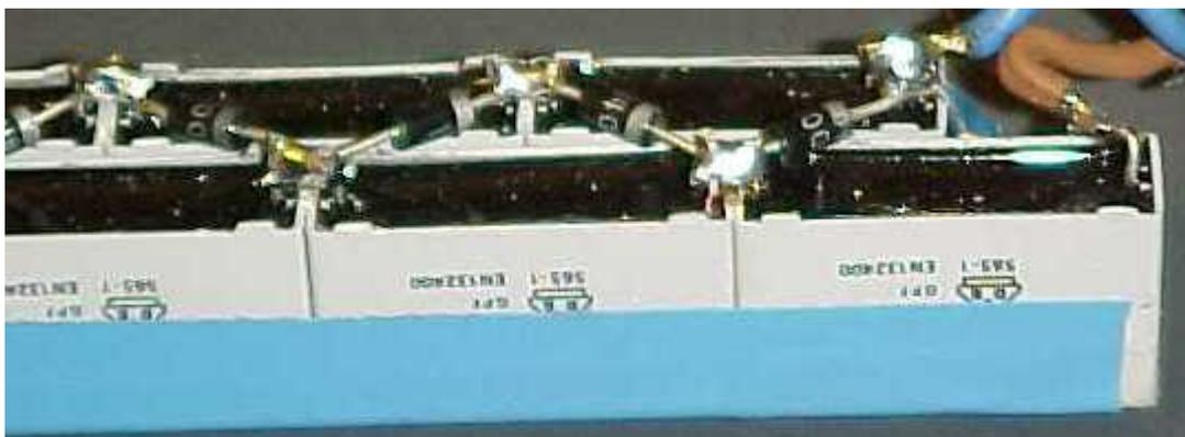
This is the mains end of a multiplier that I hard wired together using 30 220n capacitors. If you attempt to assemble your own multiplier in this manner, then be careful to tin all the connections with solder before assembling them since soldering four loose connections together can be quite awkward, even when the capacitors have been stuck together rigidly.
