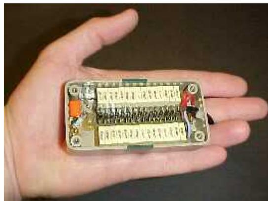
A kit ioniser from many moons ago. This neat design packs a lot of ioniser into a very small space, but compromises on electrical separation in doing so.
