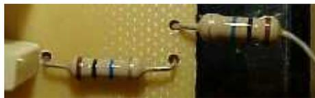
Here's a close-up of the safety resistors between the voltage multiplier and the output needles.
