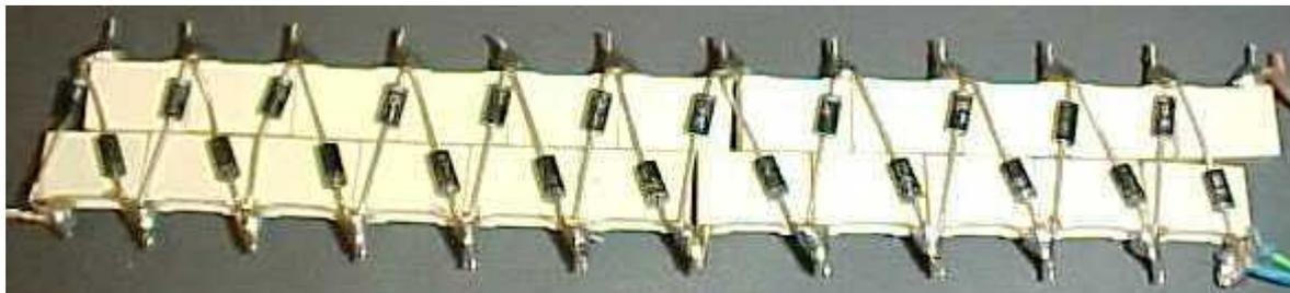
Modern versions of the same brand and many other brands have ditched the circuit board completely, and just hard-wire the components together like this. This approach to manufacture makes the circuitry much cheaper and has significant advantages of isolation between high voltage parts.
