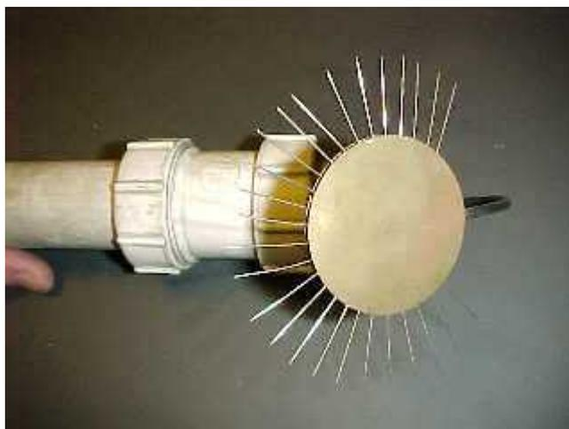
Commercial ionisers have to shield their emitter needles for safety and this can affect their output by restricting the airflow in the vicinity. But this home built ioniser doesn't suffer from this restriction!
