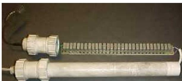
This on the other hand is a PCB based voltage multiplier built with 30 100n capacitors some time ago. It was fitted into a piece of drainage piping and used as a powerful ioniser.
