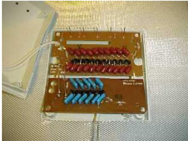
This rather interesting variant on a normal ioniser has two voltage multipliers. The red one generates the high negative ionisation voltage, while the blue one generates a much lower positive voltage which is applied to a metal mesh on the base.
