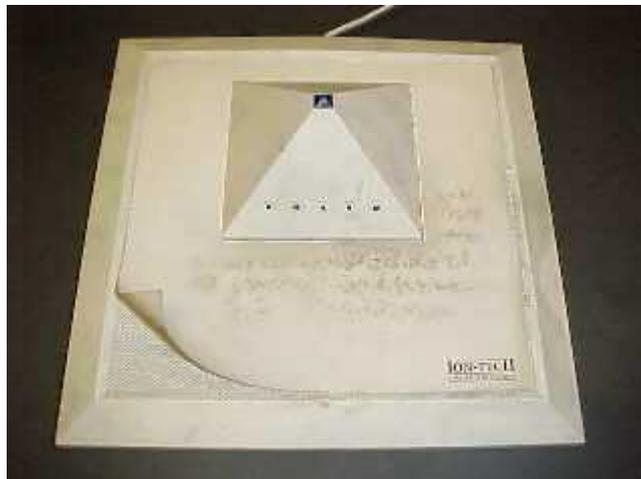
The mesh on the base is then covered with disposable paper mats, and the fact that it is at a lower potential than the natural ground means that the negatively charged dust tends to gather on the paper instead of the surrounding furniture. (theoretically)
