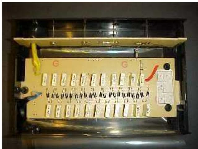
It was sealed too, but one quick crack with a screwdriver and it popped open nicely. It uses the standard layout of 10n caps, IN4007 diodes and two 10M resistors connected to a cluster of needles. Most ionisers of this type tend to use only about 22 capacitors since they seem to regard this as the minimum they can get away with. This is possibly to keep the ozone emissions from the needle corona low, but is more likely to keep the cost of manufacture down!
