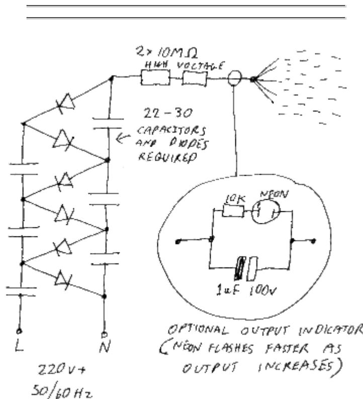
This is the basic circuit of most ionisers. It's basically a long Walton Cockroft style voltage multiplier running directly from the 220/240V mains supply, which has it's high voltage output applied to the emitter needles via a couple of high voltage high value
